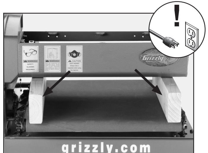
Figure 44. Gauge blocks placed under drums.
